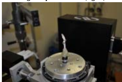
Fig. 2. Micro-CT investigations using the Synchrotron Radiation at the SYRMEP Beamline of the ELETTRA Synchrotron Radiation Facility (Trieste, Italy)
